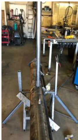
Yardarm fabrication in progress
